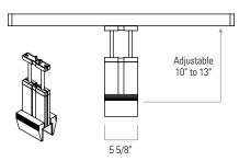
Expandable Bracket This adjustable bracket clamps onto furniture systems ranging from 2" to 4" thick.
